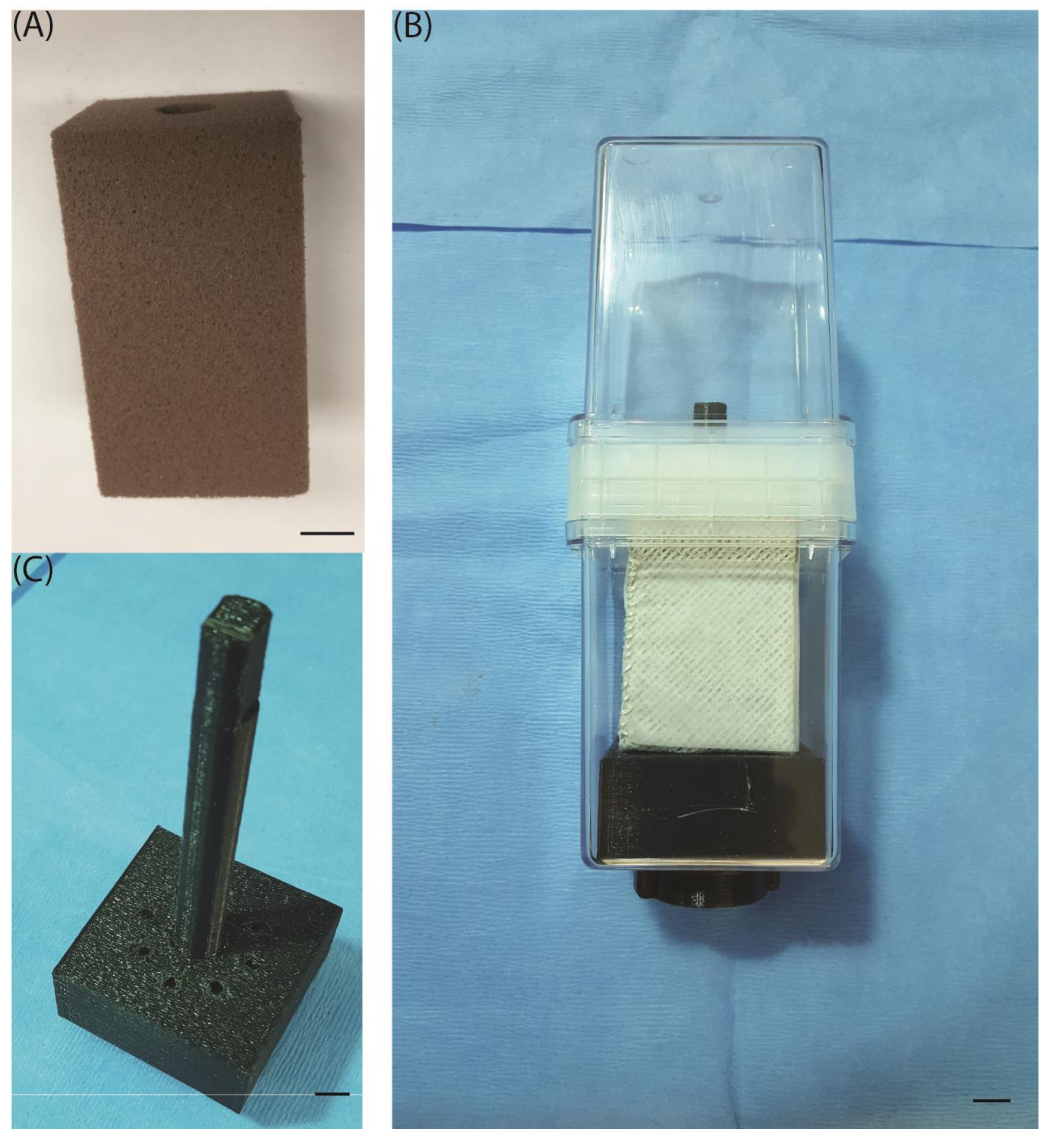
Figure 1. The APEX Growth Unit hardware. (A) The central Oasis Hortcube foam block (LC2, Oasis Grower Solutions) is used as a seed support during takeoff as well as following germination. It also serves as a nutrient reservoir during seedling growth. (B) The fully assembled APEX Growth Unit contains a foam block wrapped with a layer of medical gauze, allowing a more homogenous distribution of growth medium at the surface of the block where germinating seedlings are located. An outer layer of Nitex mesh prevents the roots of germinating seedlings from penetrating into the foam block, thereby hindering observation of their growth. (C) A growth-medium injection showerhead carries a central stick that serves as a support for a foam cube within the Magenta box. The injection showerhead is accessible for nutrient injection into the foam block through a port that crosses the Magenta box wall at its bottom. Black lines refer to 1 cm.
